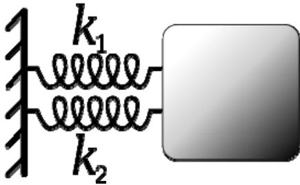
Two springs attached to a wall and a mass. In a situation like this, the two springs can be replaced by one with a spring constant of  $k_{eq}=k_1+k_2$ .
